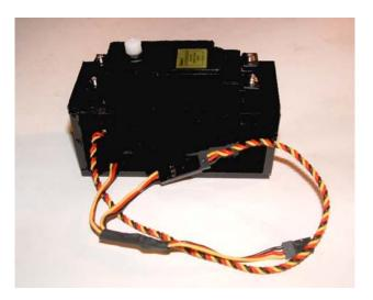
Step 5: <u>Servo Assembly Installation:</u> Install the servo assembly by gluing the servo mount to the main gun barrel within the turret. Use scrap ABS to provide a level base for the servo mount. Install the assembly with the servo output shaft located towards the back of the turret. The servo output shaft should also be located approximately ten inches from the main gun pivot, which is located at the front of the turret.
