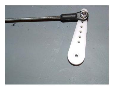
**Step 8:** <u>Servo Rod Forming:</u> Form a "V" in the connection rod. This "V" provides some protection to the servo in the event that the gun barrel is obstructed from movement during elevation change. Although the rod shown below has a ninety degree bend, the exact location of this bend has to be customized for each servo assembly installation. This will be covered in the following step.
