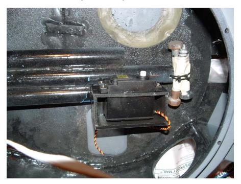
**Step 6:** Fixed Servo Arm Installation: Install the fixed servo arm to the turret. The fixed servo arm is fitted to the inside of the front of the turret. The fixed servo arm should be slightly offset from center, so that it will be in line with the moveable servo arm at the servo. Glue the ABS fixed servo arm to the turret. Use a small piece of the ABS scrap material as a fillet brace for the fixed servo arm.
