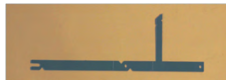
(2) Upper Deck (Hull) Side Shield Bracket (Rear) bra001-S526M
